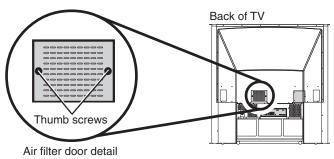
NOTE: The air filter door is provided with an interlock to reduce the risk of damage to the TV. Do not defeat its purpose or attempt to service without removing the door completely.
